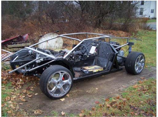
Pic #53 Side view showing roll cage etc.
