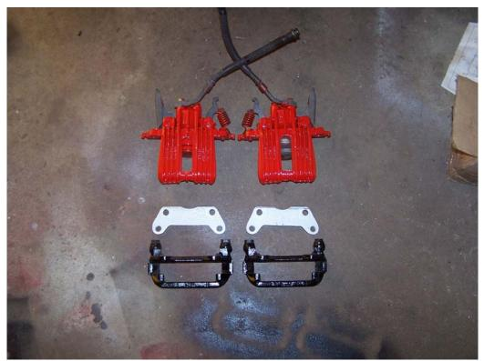
Pic #50. Here we have the C-4 Corvette rear calipers and custom mounting brackets for the Cadillac rear struts.
