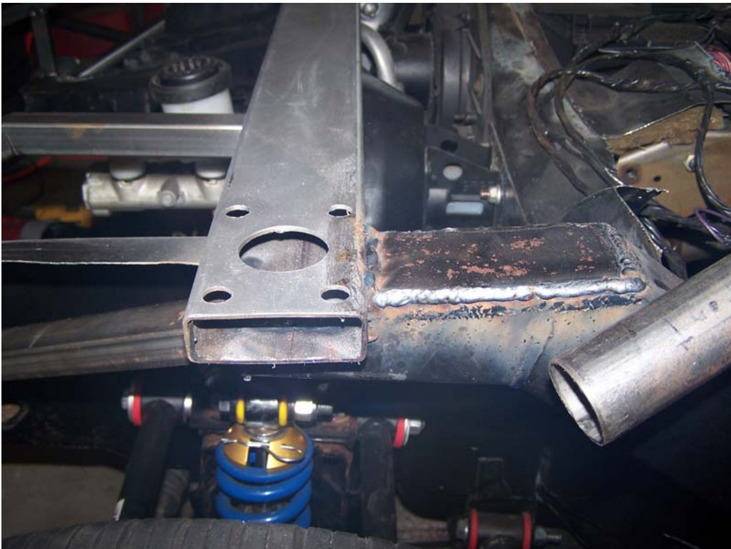
Pic #39 After dropping the brake booster 3/4" along with lowering the A/C accumulator, I mounted the windshield/door hinge support bar.
