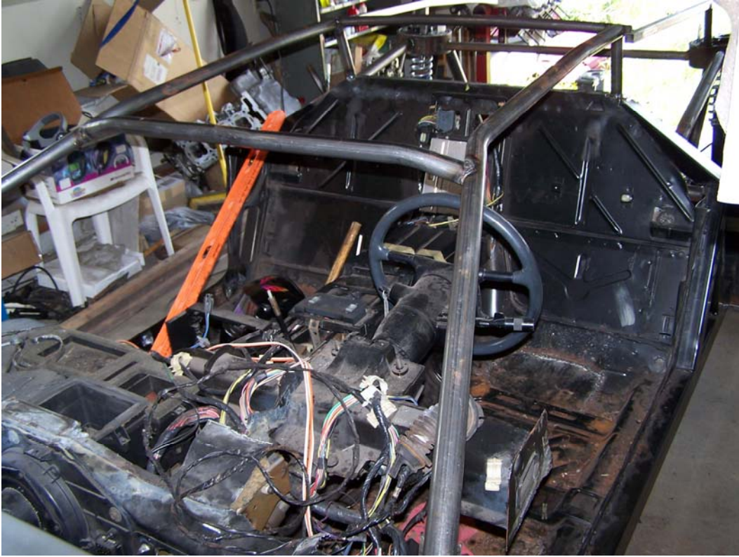
Pic #42 This picture shows the upper cage tubing for strength of the chassis.
