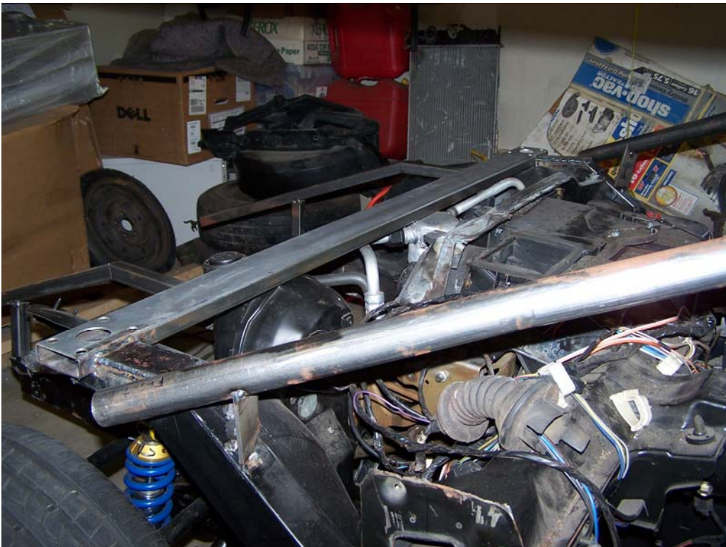
Pic #41 Picture shows the area where the upper body support tubing attaches to the left side of the windshield area.
