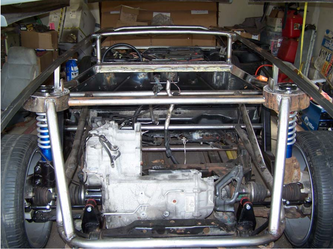
Pic #44 Here we have a shot of the rear framework tubing.
