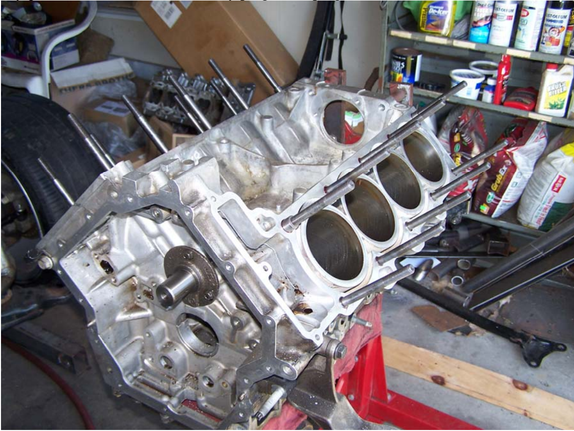
Pic #37 While rebuilding the Cadillac Northstar, I installed head studs into the block to keep the heads on tight.
