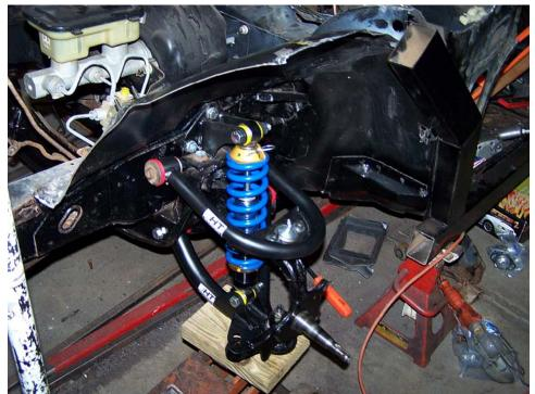
Pic #27 - Back to working on the "beast". I modified the left front and right front upper spring perch per instructions from HT Motorsports (Held Suspension) and then installed the Wide Track coil-over suspension on the left side.
