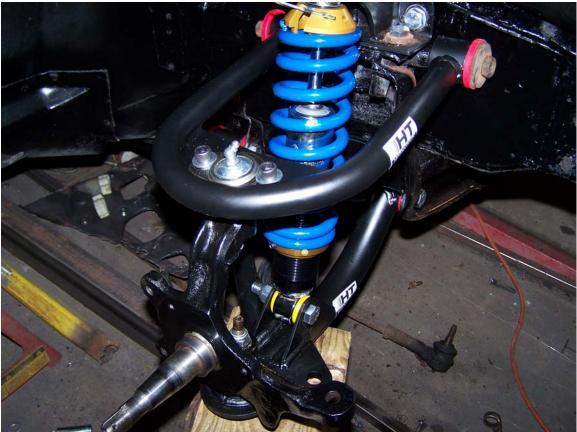
Pic #28 - This picture shows the right front side suspension installed. The HT Motorsports Wide Track Kit is fairly easy to install. Taking off the old a-frames can be tricky. Safety first kids.
