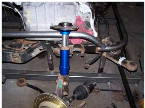
Pic #20. The Cadillac strut has had the lower spring seat removed along with the torsion bar link bracket so that the Mustang Coil-over tube can be installed. Slight modifications were made to the Mustang kit for it to work on the Cadillac strut. A spacer tube was cut to a length of  $3\frac{1}{2}$ " and installed on the strut shaft to simulate the mid ride travel height of the strut to properly locate the strut cap position for welding.
