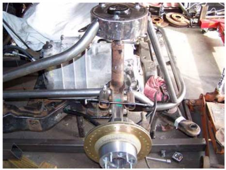
Pic #22. This pic shows my little strut alignment jig to hold the strut vertical. It was attached to the tube frame with two muffler clamps and was adjustable and worked well. The cap has been tack welded in the correct position before final welding.
