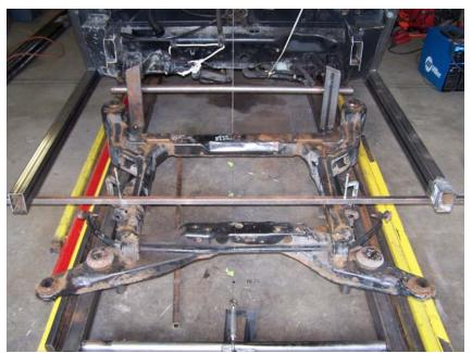
Pic #14 Rockers all welded and ready for more cutting and welding.
