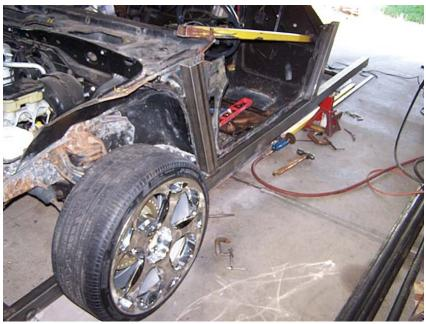
Pic #17 Body has been centered on floor jig and welded solid utilizing the rear cradle mounts on the firewall. Cadillac cradle has been centered and aligned to the rear wheel centerline. It is spaced 5½" ground clearance. Now comes the fun of building the tube framework.
