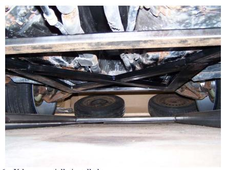
Pic #16 X-brace partially installed
