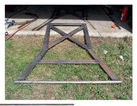
Pic #13 Slightly modified X-brace for Body strengthening after rocker reinforcements are welded in.
