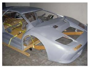
Parts strapped inside of body shell. Note front support arms. Same design for rear support arms, to minimize vibration and bounce on body during transporting.
