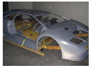
Note the side bumper rails (2" X 3" board) that extend 1 ½" past body and keeps the body from hitting sides of freight vehicle. Tie-downs secured for the trip.
