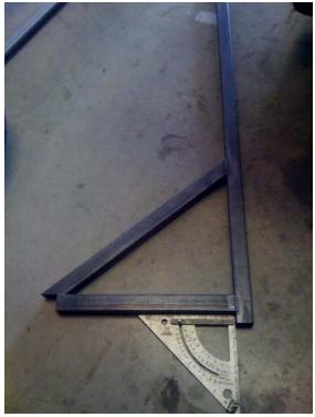
Fabricating chassis modification parts
