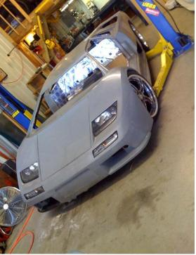
I still need to finish up the body work. But here Is a rough look at the finish product. As you can see I'm still working on the carbon fiber lower pieces. I'm making a mold next week to fabricate better looking pieces.
