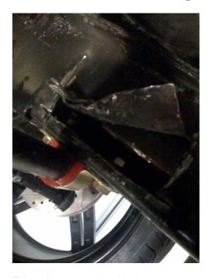
This took me some time. I had to cut a opening on both sides of the frame rails to have access to the old nuts that were welded in there. I drilled the old bolts and nuts and replaced them with new grade 8 bolts. I will soon weld everything shut. Will look like factory again but better! The reason this happened was the old bolts holding the bushings brackets all 4 broke while I was taking them out. That lead me to drilling them and going thru the above process.
