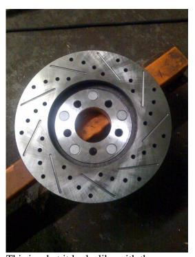
This is what it looks like with the adapter mounted inside of the rotor
