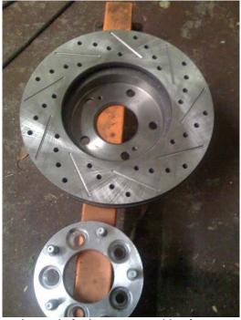
Instead of adapter on outside of rotor...now it's hiden inside the rotor. Now I still gained that 1 inch. With invisible appearance of the adapters!
