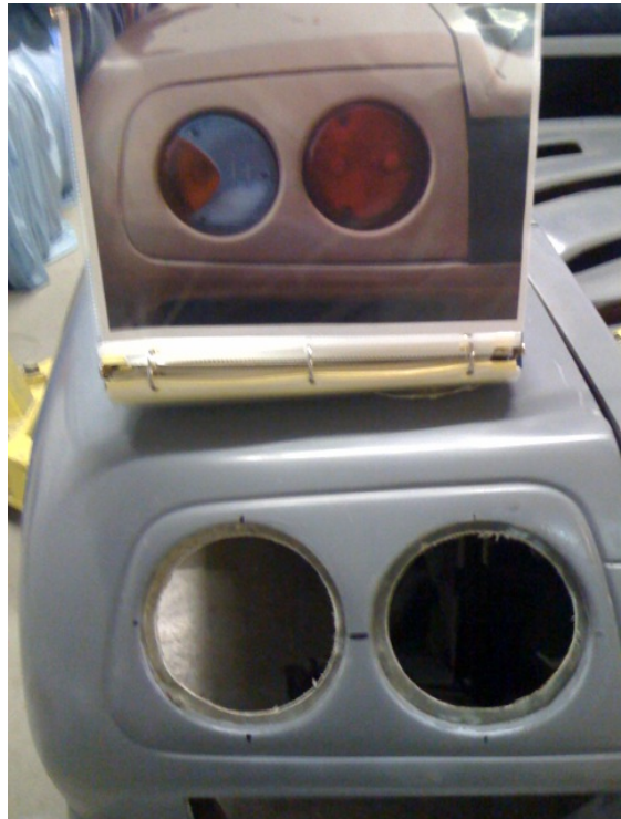
Holes cut in molded mounts as per picture Diabolic with molded in taillight holes
