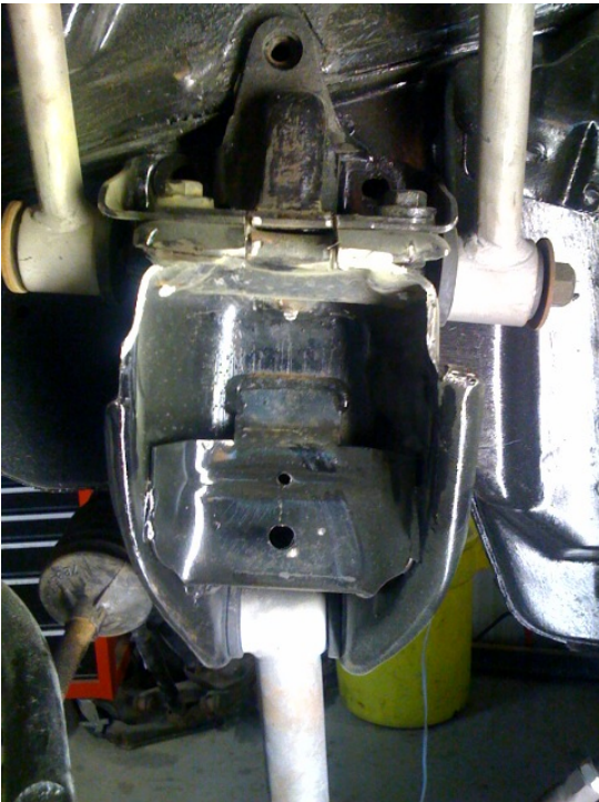
New control arms and A-Arms installed for wider tracking
