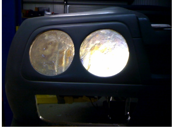
Fiberglass was molded over the openings to prepare for smaller holes required.
