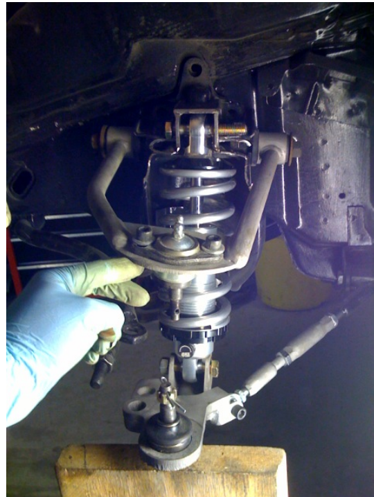
New control arms and A-Arms installed for wider tracking
