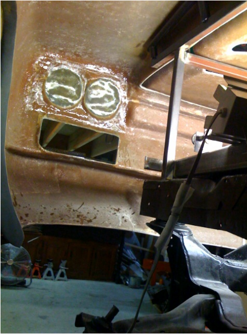
Fiberglass was molded over the openings to prepare for smaller holes required.
