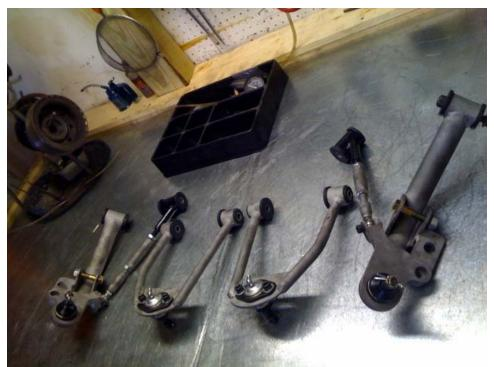
Modifying the suspension for proper tracking and A-frame length. Here we are receiving the replacement suspension parts to be installed for proper tracking.
