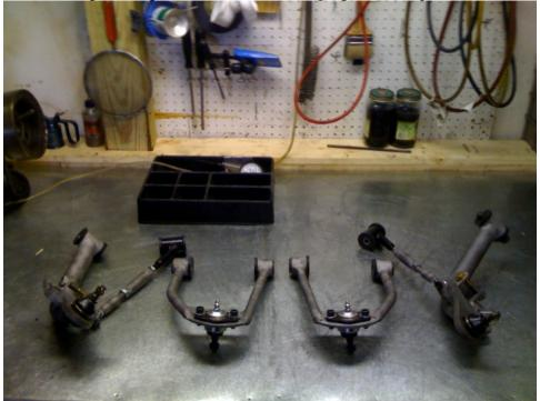
Felipe had these suspension components custom modified. The custom suspension parts are definitely a better choice than wheel spacers. The offset of the rims must also be taken in consideration when designing.
