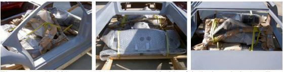
The paper and bubble wrapped parts are secured inside of the body to the body pallet with ratchet tie downs.
