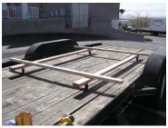
The body is lifted on the trailer and the short range body pallet is inserted under the body and secured in 4 corners with screws and fender washers.
