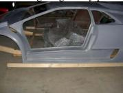
There are now a total of (4) of the 2" X 3" X 77" boards going across. Front and rear support struts are added with 3 lag bolts on each strut to secure each. There is also a "protective bumper board" added on each side of the body.
