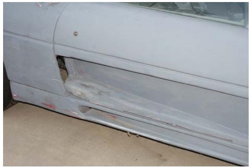
These door panels were very rough and damaged, requiring fiberglass cloth and filler to be added to buildup the surface as it should be. Notice the before shot above.
