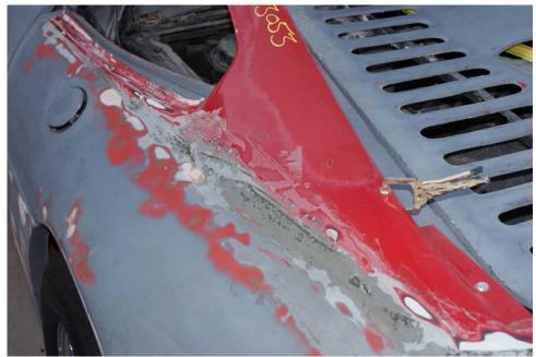
Adding the rear section from a Fiero GT, cutting it to fit, and molding it in, definitely makes the car look more like the Ferrari F355 coupe.
