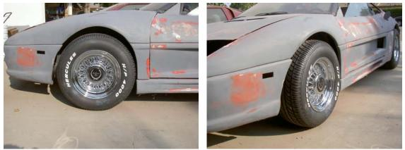
The front has P245-60R15 tires mounted on 8" X 15" wheels. The simulated spoke baskets are installed to give a more realistic look. Definitely an improvement.
