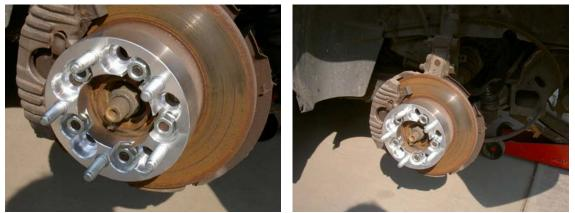
A combination adapter/spacer was installed on all 4 hubs to allow the different lug patern rims to be mounted.
