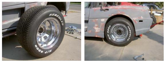
The P295-50R15 tires were installed for the back on 10" X 15" rims
