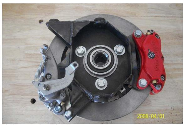
Disk brake assembly on spindle plate
