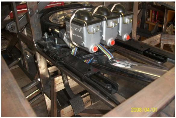
Clutch and brake cylinders above moveable pedal assembly
