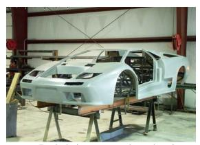
Body being mounted on chassis
