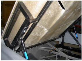
Fabricating engine hatch mounting
