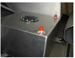
1 of 2 fuel cells to be installed
