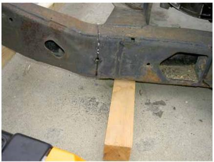
Prop the cradle on blocks to allow clearance for the saw to cut.
