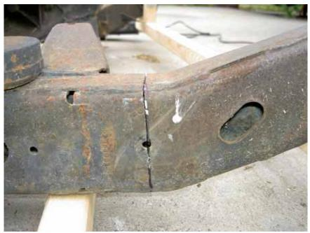
Saw both sides nearly thru to bottom.
