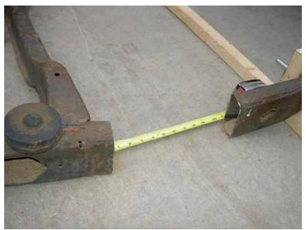
Check 3 or 4 times to make sure both sides are  $10 \frac{1}{2}$  separation.
