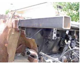
Making sure the chassis is level. Making sure the cradle is level. Making sure the upper extension tubes are level. Now the rear portion of the vehicle may be moved up and aligned to the extension tubes. The lower tubes will have to be pounded into the frame rails.
