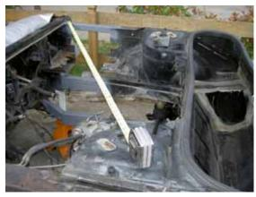
Once you have exactly 10 ½" (3" for F355, 7" for Countach) in between the front and rear frame cuts check for level again. Measure from the strut tower center hole diagonally over to the firewall opposite outer corner. The cradle frame should be able to be bolted back to the upper frame at the rear mounting points. This will help secure the alignment.
