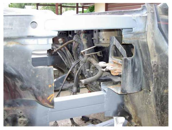
Extension tubes welded in on passenger side. Note that sheet metal can be added back in to cover the  $10 \frac{1}{2}$ " opening created by the extension.
