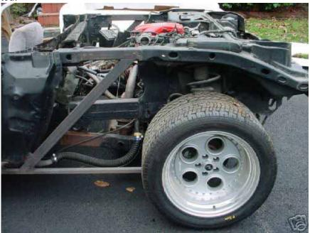
It is necessary to weld a 1" x 2" piece of tubing at a 45 degree angle from the lower rocker panel area up to the rear portion of the stretched section (on both sides). Now take a deep breath . . .
