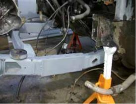
The cradle should be put on jack stands and leveled. The level can be placed on the cradle extension tubes. Using a hydraulic jack under the rear of the swing arm allows minor movements to level it.
