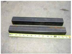
Use square tubing to extend the frame rails. Top=1  $\frac{3}{4}$ " x 1  $\frac{3}{4}$ " x 14 $\frac{1}{2}$ " in length / Bottom=(2) 1  $\frac{3}{4}$ " x 14 $\frac{1}{2}$ " in length with 1/8" wall thickness (F355 uses Top =1 $\frac{1}{2}$ " x 2" x 7" in length / Bottom= (2) 1 $\frac{1}{2}$ " x 2" x 7"). The bottom frame rail requires two pieces of square tubing stacked one on top of the other for added stability.
