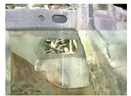
Driver Side Passenger Side Be sure to mark all the way up and down on both sides that are to be cut.
