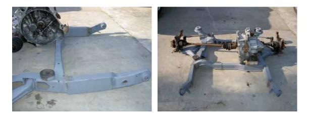
Metal reinforcement plates must be welded over the extension tubes for better strength.
