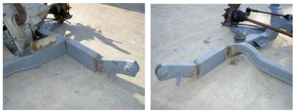
If all alignment is proper, securely weld the cradle extension tubes in place.
