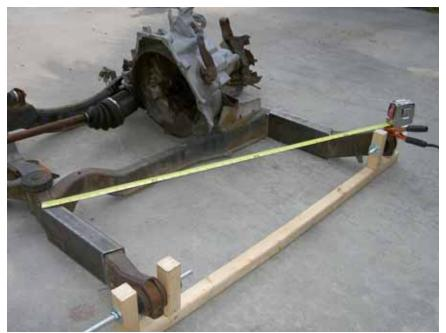
With the parts laid out, check for alignment and symmetry
