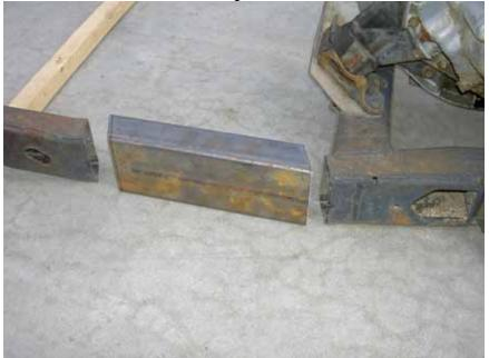
This is the stretch tube for the cradle (2 required) shown here on the driver side. These are available from B and B Customs. www.BandBCustoms.com
