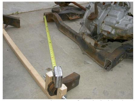
Take a tape measure and measure from the inside edge of the passenger side of the cradle to the center of the mounting bolt on the drivers side of the swing mount (39 1/4" was found in our case).
