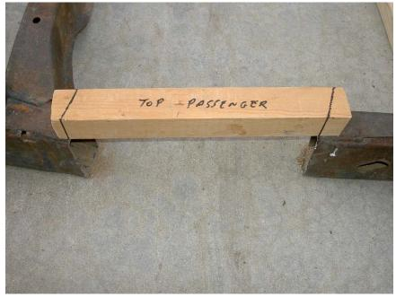
Flipping the block over should be a perfect fit for the passenger side. Once the block is marked, you can cut it to use as a template.
