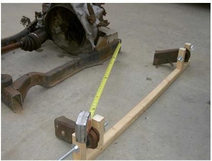
Now do the same but measuring from the drivers inside of the cradle to the center of the mounting bolt on the passenger side. This distance should be the same as the previous measurement (again  $39 \frac{1}{4}$ " in our case). Check this measurement both ways 3 or 4 times and move it slightly if not identical until both match perfectly. Remember to keep the space between the cut surfaces at  $10 \frac{1}{2}$ ".
