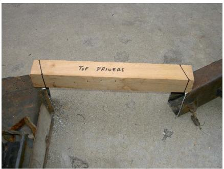
Laying a block on top of the surfaces, and using a felt pen, you can mark the angles on the bottom of the block to use as a future template. With a square, draw lines up each side. Finally connect the lines across the top of the block. Mark the block for the side it will fit, and mark the opposite side for the other.
